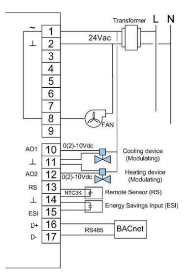
Wiring: 14 to 22 AWG wires or 1.5mm<sup>2</sup> wires.
